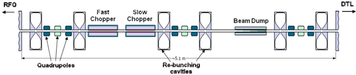
Figure 3: Schematic drawing of the MEBT Scheme 3.
