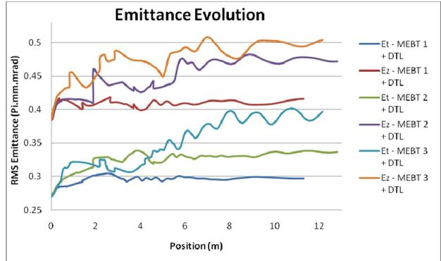
Figure 5: Longitudinal and transverse (average Ex and Ey) emittance evolution (Normalized RMS) for the three MEBT schemes and the DTL.
