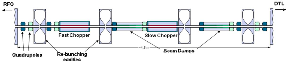
Figure 1: Schematic drawing of the MEBT Scheme 1.
