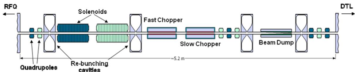
Figure 2: Schematic drawing of the MEBT Scheme 2.
