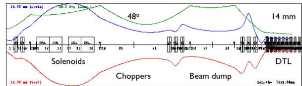
Figure 1: The beam amplitudes through the MEBT unit.
