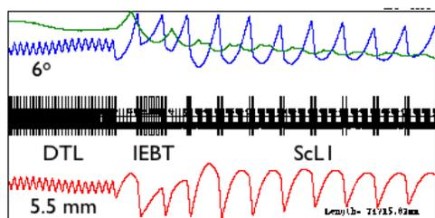
Figure 2: Beam amplitudes over the IEBT transition.
