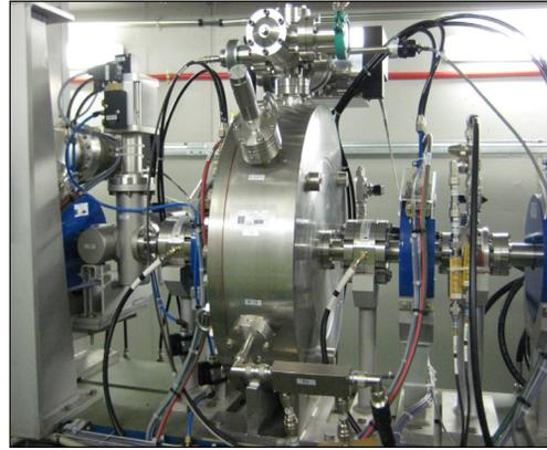
Figure 1: Prebunching cavities and shielded lenses.
