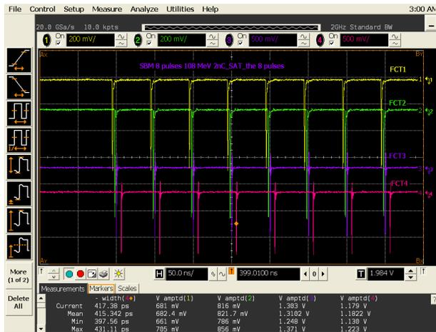
Figure 3: FCT signals for the SBM mode.
