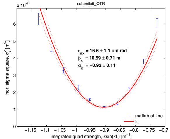
Figure 5: MBM horizontal emittance measurement.
