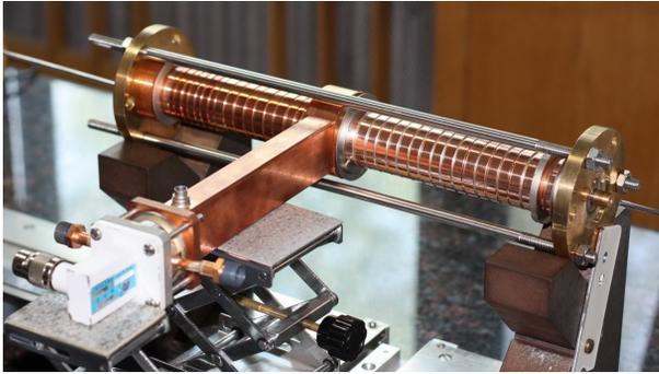
Figure 3: 4MeV X-band accelerating tube assembly
