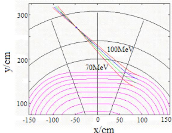
Figure 2: Extracted trajectories for 70 MeV, 80 MeV, 90 MeV and 100 MeV particles.
