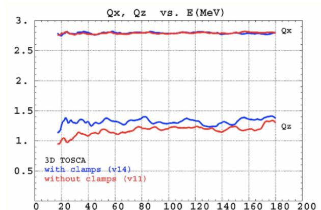
Figure 2: Horizontal and vertical tunes versus kinetic energy in two models : with and without field clamps.
