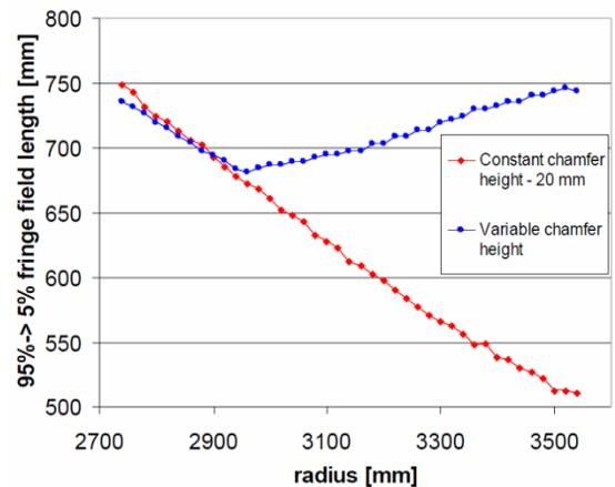
Figure 1: Total fringe field length in two models : with and without variable chamfer.
