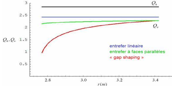
Figure 3: Tunes for various gap shapes in the model FFAG-spi [5].
