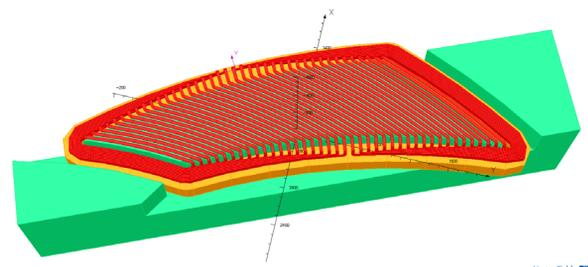
Figure 6: 3D model. Distributed conductors in red, main coil in yellow.
