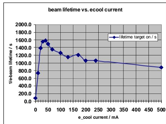
Figure 3: Beam lifetime as function of electron beam current. At low current the beam is not sufficiently cooled, therefore the beam lifetime is short. At large electron beam current the proton beam lifetime is reduced as well.
