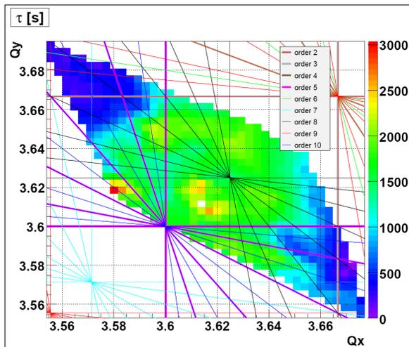
Figure 5: Beam lifetime as function of horizontal and vertical tunes  $Q_x$  and  $Q_y$ , respectively. The lines are the betatron resonances up to order 10. Longest beam lifetime is achieved at around  $Q_x = Q_y = 3.61$ .
