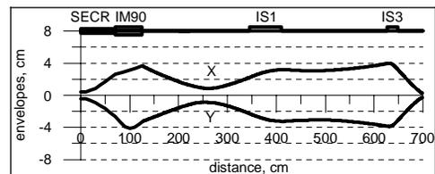
Figure 2: Horizontal (X) and vertical (Y) beam envelope.
