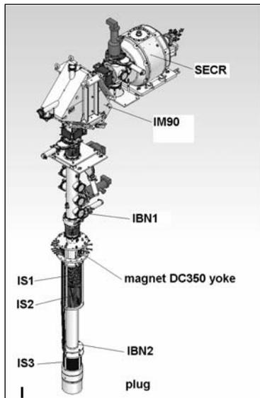
Figure 1: DC350 axial injection channel layout.
