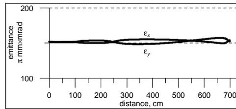
Figure 8: Horizontal ( $\epsilon_x$ ) and vertical ( $\epsilon_y$ ) beam emittance (after correction).
