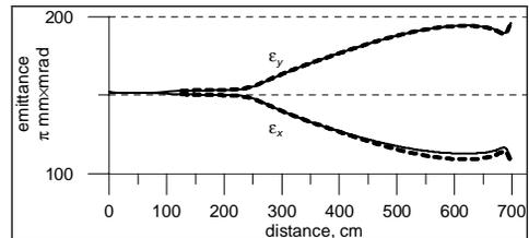
Figure 5: Horizontal ( $\epsilon_x$ ) and vertical ( $\epsilon_y$ ) beam emittance.
