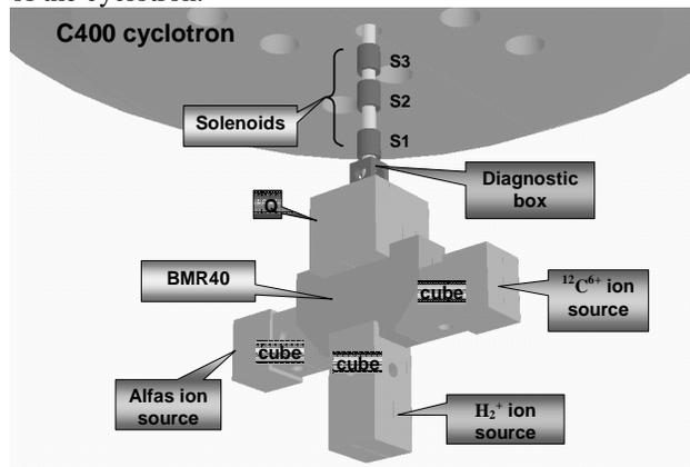
Figure 1: C400 axial injection beam line
