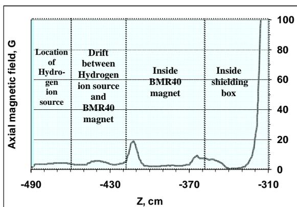
Figure 5: Axial magnetic field distribution on vertical axis of C400.
