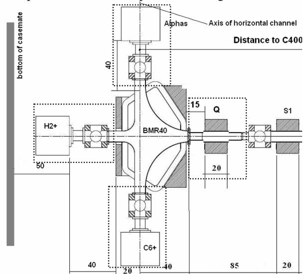
Figure 3: The scheme of the axial injection beam line and regions of an additional shielding (dashed lines).
