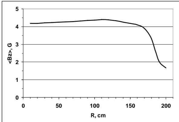
Figure 8: Dependence of the average magnetic field in MP on radii.
