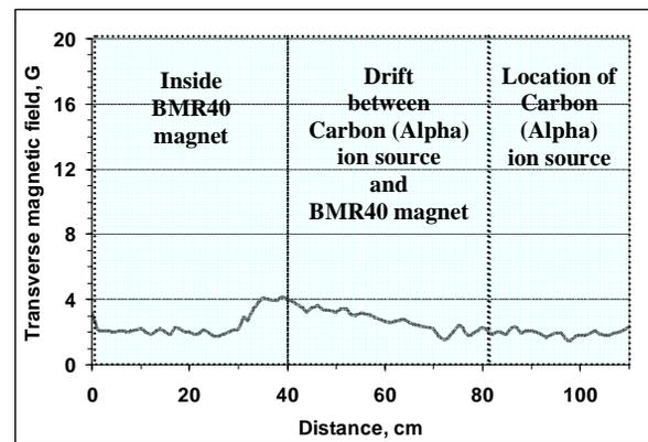
Figure 7: Magnetic fields along horizontal beam line.
