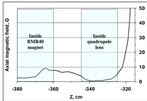
Figure 6: Axial magnetic field distribution on vertical axis of C400. Fragment.
