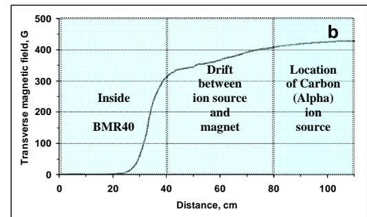
Figure 2: C400 magnetic field distributions in the region of the injection beam line elements
