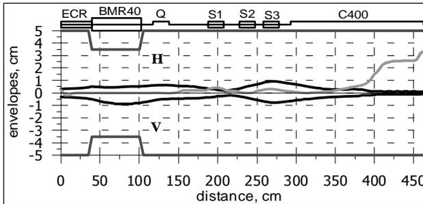
Figure 7: Horizontal (H) and vertical (V) envelopes of  $\text{He}^{2+}$  ions beam.
