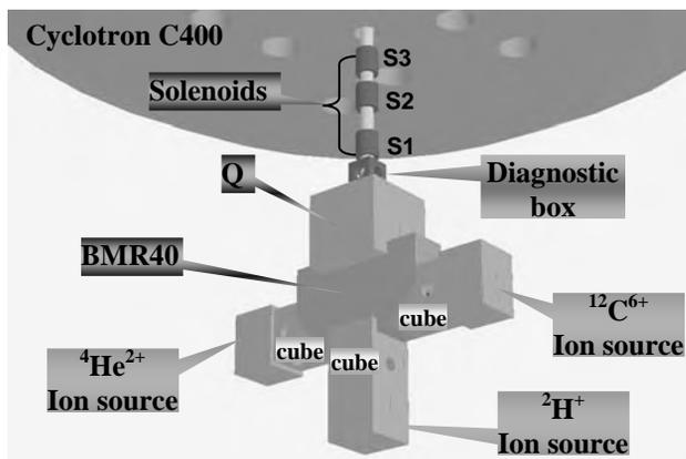
Figure 1: C400 axial injection beam line.
