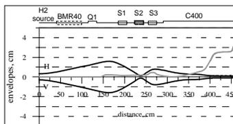
Figure 9:  $^2\text{H}^+$  ions beam envelopes.
