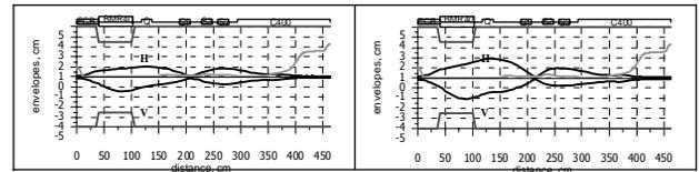
Figure 4: Horizontal (H) and vertical (V) envelopes of  $\text{C}^{6+}$  ions beam.  $f=1$  – left,  $f=0$  – right.
