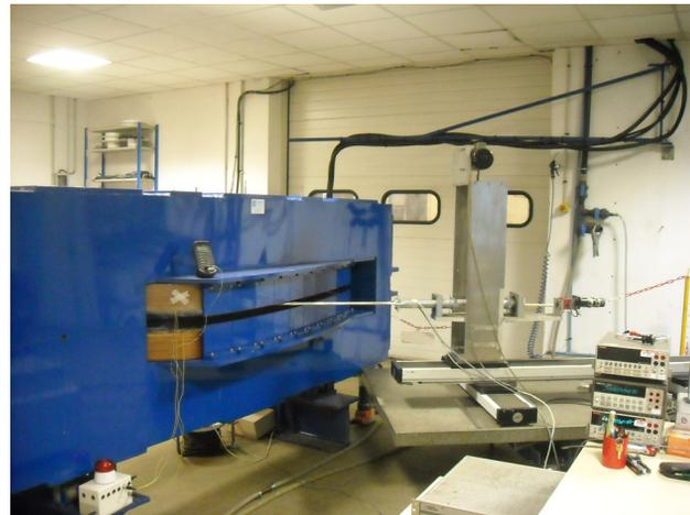
Figure 5: Magnet, mapping table and Hall probe system.
