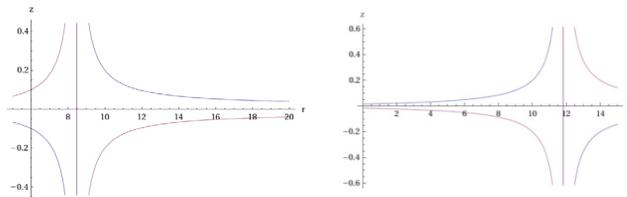
Figure 1: Pole shapes: focusing (LHS), defocusing (RHS). The asymptote denotes the lower and upper range, respectively, for which stable orbits may be found. Blue and red lines denote north and south poles, respectively.  $B_0 = -5$  Tesla,  $B_1 = \pm 5$  T/m and  $r_c = 10$  metre.
