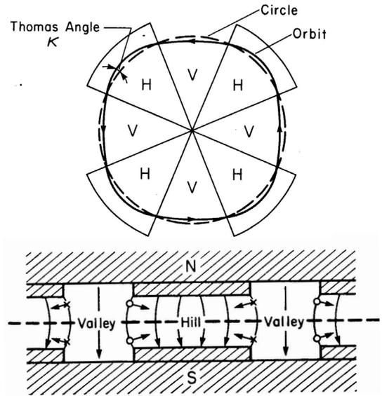
Figure 3: A radial-sector cyclotron, showing orbit scalloping and the Thomas focusing at the sector edges.
