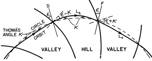
Figure 4: Edge crossing angles in a spiral-sector cyclotron.
