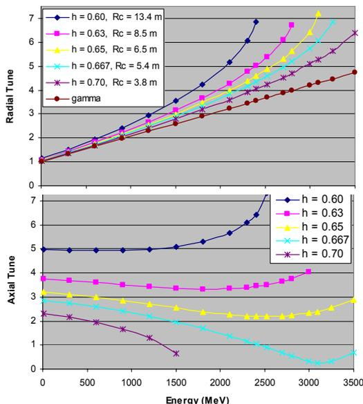
Figure 4: Tunes in a reverse-bend cyclotron with constant fields on orbit ( $N = 15$ ,  $h$  and  $R_c$  as shown).
