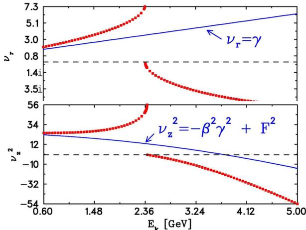
Figure 3: Tunes in a reverse-bend cyclotron with constant fields on orbit ( $N = 15$ ,  $h = 0.6$ ,  $R_c = 15.65$  m).
