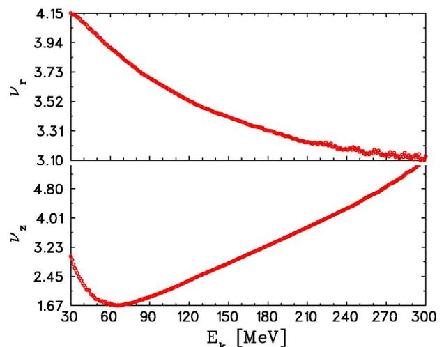
Figure 1: Tunes in the tune-stabilized medical FFAG computed by CYCLOPS.
