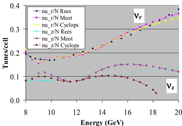
Figure 2: Betatron tunes in the isochronous IFFAG, as computed by Rees, Méot and CYCLOPS.
