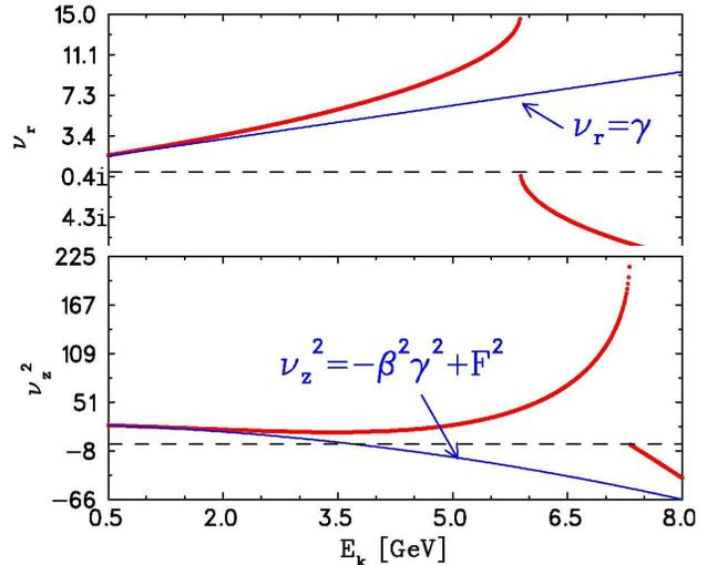
Figure 5: Tunes in a reverse-bend cyclotron with constant fields on orbit ( $N = 15$ ,  $h = 0.6$ ,  $R_c = 15.65$  m).
