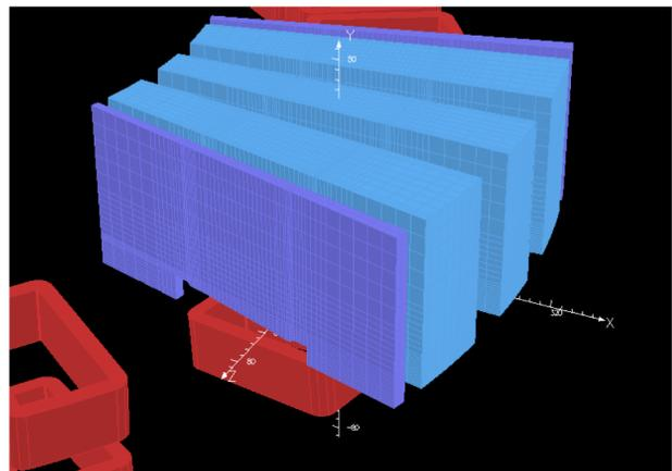
Figure 2: A 3D model of the FFAG-ERIT magnet.
