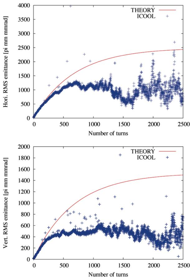
Figure 3: Transverse and longitudinal emittance growth in ERIT.
