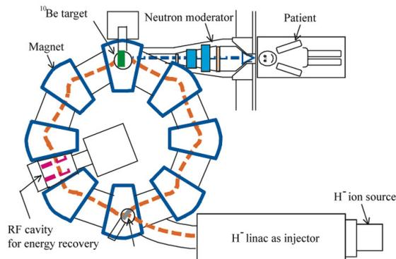
Figure 1: A schematic layout of ERIT scheme.
