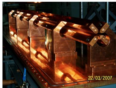
Figure 3: The 3.4m RFQ post-accelerator.
