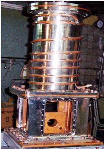
Figure 4: The Re-buncher during assembly.
