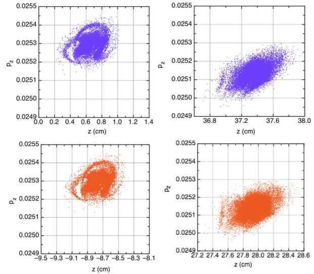
Figure 7: Longitudinal particle distribution before (left) and after (right) funneling.
