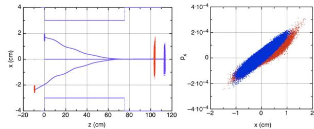
Figure 9: Funneling of 300 keV/u  $^{238}\text{U}^{33+}$  beams in modified 40 MHz RFQ.
