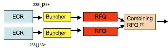
Figure 8: Beam funneling based on combining RFQ.
