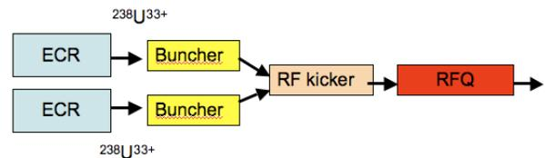
Figure 1: Schematic layout of funneling of bunched beams extracted from ECR sources.
