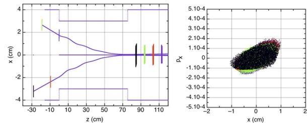
Figure 10: Funneling of two charge state bunches: (blue, red)  $^{238}\text{U}^{33+}$ , (green, black)  $^{238}\text{U}^{34+}$ .
