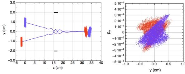
Figure 3: Funneling of  $13.8 \text{ keV/u } ^{238}\text{U}^{33+}$  beams in RF kicker. The beam oscillation outside the kicker are produced by the fringe fields.
