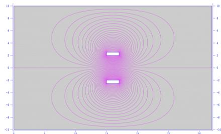
Figure 2: Field distribution in RF kicker for beam funneling.
