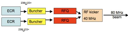
Figure 4: Beam funneling with post-RFQ kicker.
