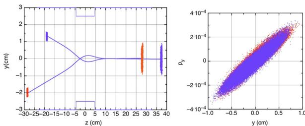
Figure 5: Funneling of  $300 \text{ keV/u } ^{238}\text{U}^{33+}$  beams in  $\lambda/2$  RF kicker and final beam overlapping.
