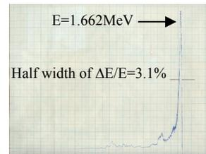
Figure 7: beam energy spectrum of experiment.
