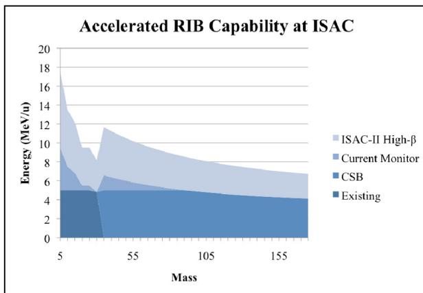
Figure 2: Progression of accelerated beams at ISAC as a function of mass. As each infrastructure improvement is implemented, higher energies become available.
