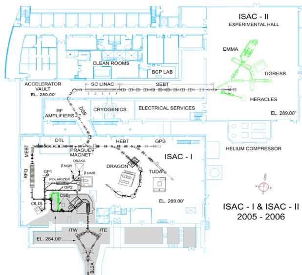
Figure 1: Plan view of the ISAC experimental halls. Protons strike one of two targets on the lower level (gray area). RIBs are mass separated before coming upstairs into the low-energy area; the RFQ and DTL accelerators serve the ISAC-I medium energy area; and the superconducting LINAC leads to the high-energy area of ISAC-II.
