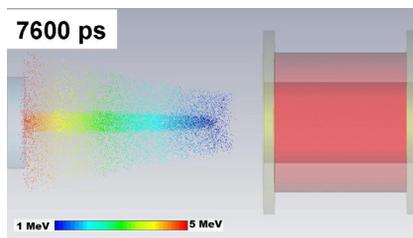
Figure 8: CST simulation: proton beam distribution behind the solenoid at  $t = 7600$  ps and a magnetic field strength of 8.6 T (including Coulomb forces). The beam comes from the right image border and goes to the RCF detector on the left hand side.
