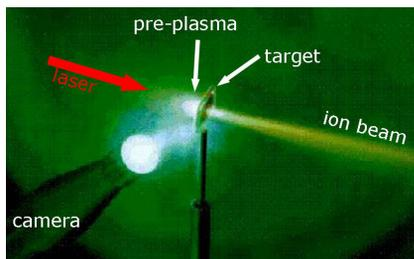
Figure 1: Photograph of the laser-ion-acceleration from a foil target at the LLNL NOVA Petawatt laser.
