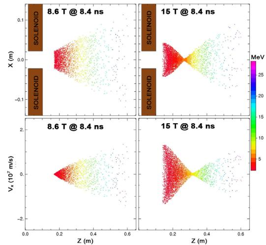
Figure 9: Warp simulations: (top) transverse deflection  $X$  and (bottom) transverse proton velocity  $V_x$  versus beam propagation direction  $Z$  for two different magnetic field strengths 8.6 T and 15 T at the time 8.23 ns. Injected proton energies: (2.3-28.7) MeV.
