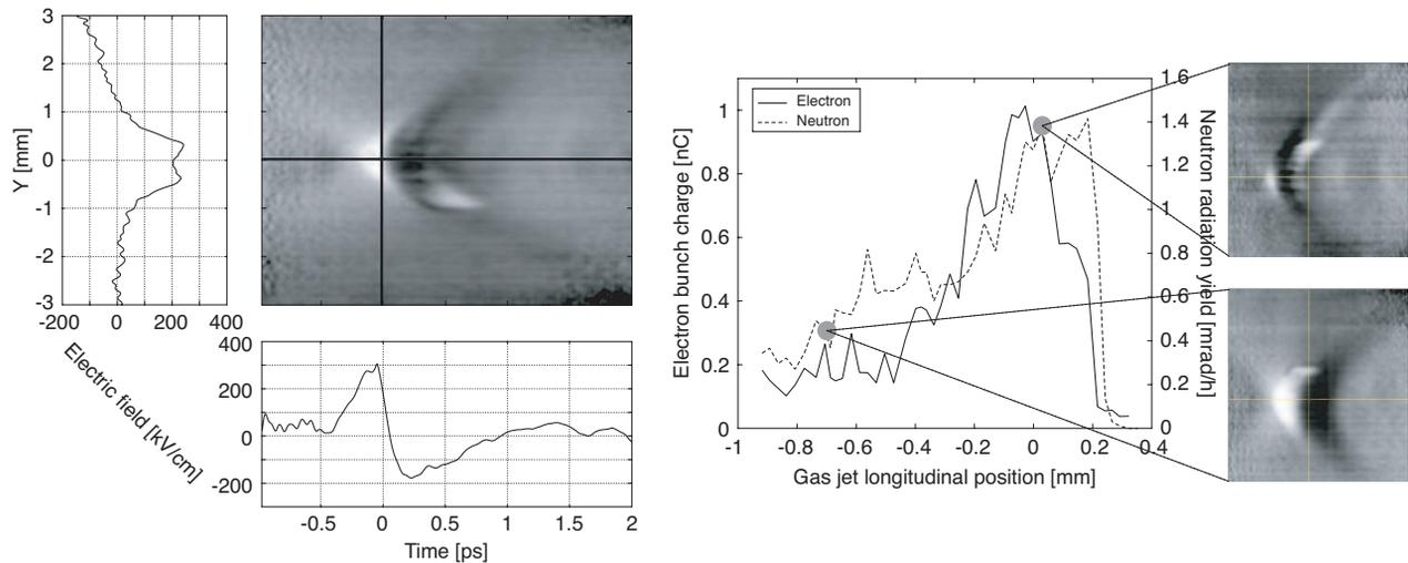
Figure 2: Space-time cross section obtained in a single-shot (*left*) by Temporal Electric-field Cross-correlation (TEX). Electron and neutron yield versus gas jet position (*right*). Spatiotemporal waveforms of the THz correlate with the accelerator performance.
