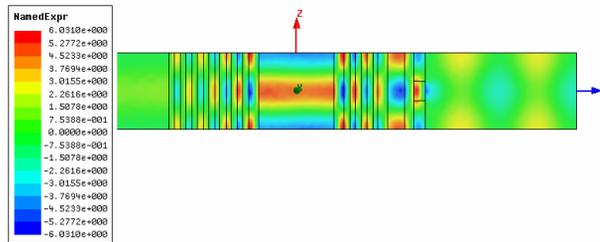
Figure 3: Field generated by prototype all-dielectric structure with a relative intensity scale (resonance: 375.2Thz). The laser enters horizontally from the right.
