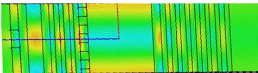
Figure 4: Fields generated by modified all-dielectric accelerating structure using GaAs and AlAs with a relative intensity scale (resonance: 374.6Thz). Laser
