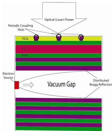
Figure 2: Schematic of the all-dielectric structure.
