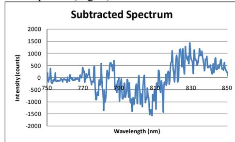
Figure 5: Laser spectrum subtracted from the spectrum of the transmitted beam through gold structure.
