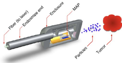
Figure 2: Conceptual representation of an encapsulated Micro-Accelerator Platform for medical applications. At one end (left), the MAP is connected to a fiber which provides the power. On the other end (right), particles are produced which are applied to destroy the tumor.
