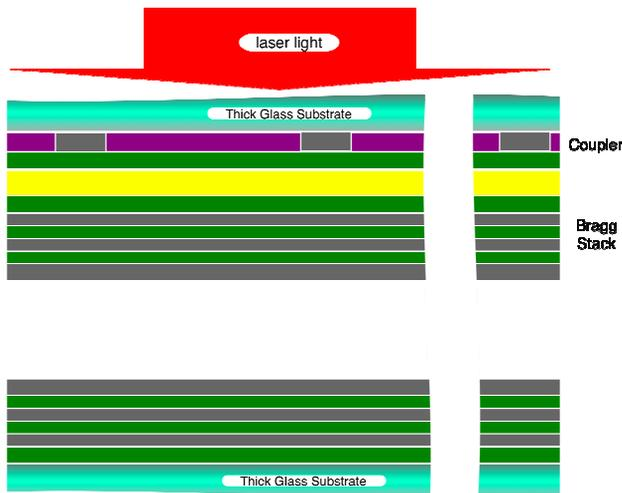
Figure 1: A cross-section of the fully-relativistic version of the Micro-Accelerator Platform.
