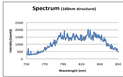
Figure 4: Transmitted Spectrum (S21) of a metallic slotted structure.
