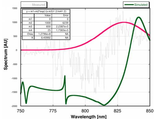
Figure 6: Simulations (green), smooth curve (pink), and data spectrum (grey) of transmitted beam through the 160nm gold structure are overlapped for comparison.
