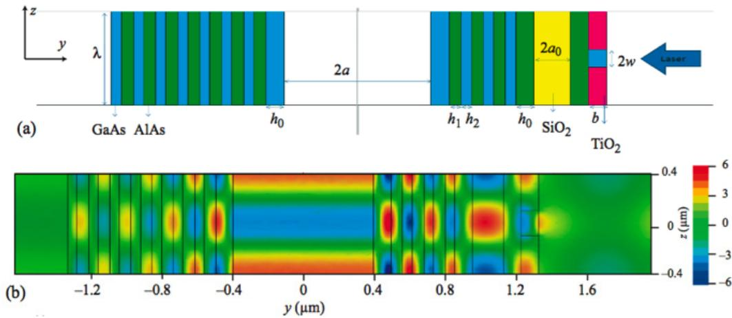
Figure 1: (a) Schematic showing the arrangement of layers and definition of parameters for one period of an all-dielectric structure. (b) False-color field map of  $E_z$  in this structure, normalized to amplitude of drive laser. (HFSS simulation). For this result,  $h_0 = w = b = 100$  nm;  $a = 400$  nm;  $a_0 = 180$  nm;  $h_1$  and  $h_2$  are  $\lambda/4$  Bragg layers.
