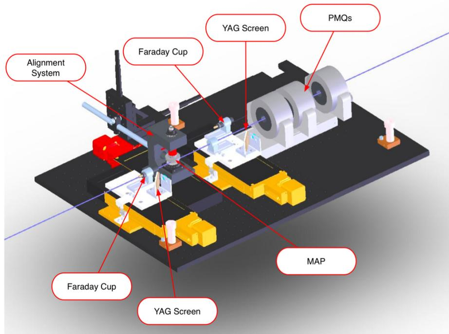
Figure 3: CAD rendering showing diagnostics and the alignment system.
