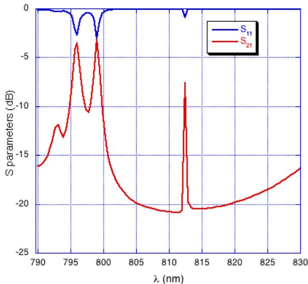
Figure 1: Simulated  $S_{11}$  and  $S_{21}$  for the dielectric structure. The desired accelerating mode is at 799.9 nm, with a weaker off-phase companion at 796.1 nm. The weak resonance at 812 nm is a non-accelerating mode.
