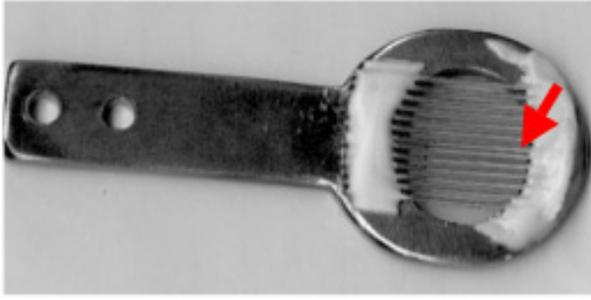
Figure 1: Picture of the wire mesh mask and frame. The wires are  $d=800\ \mu\text{m}$  in diameter with a period of  $D=1650\ \mu\text{m}$ . The red arrow indicated the two consecutive wires.
