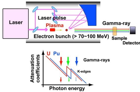
Figure 1: Schematic of tall-optical monochromatic K-edge dosimetry system.
