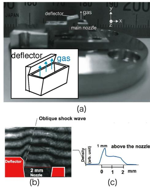
Figure 2: (a) A Photograph of the jet nozzle with a deflector. (b) Interferogram of gas jet showing a density jump produced by the oblique shock. (c) Density distribution at a distance of 1.1 mm from the nozzle exit.
