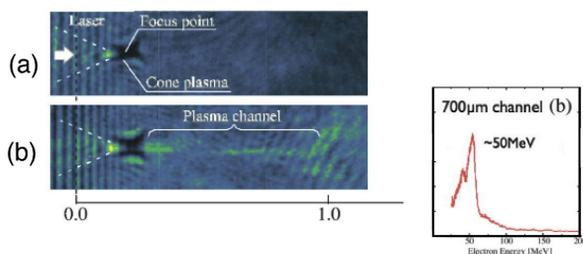
Figure 4: (a) Shadowgraph of the plasma without picosecond-prepulse in the 1-T magnetic field. (b) Shadowgraph of the plasma and the electron energy spectrum after tuning of picosecond-prepulse level in the 1-T magnetic field.
