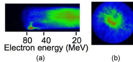
Figure 3: (a) Angle-resolved electron energy spectrum at low ns-prepulse energy. (b) Transverse distribution of electron bunch.
