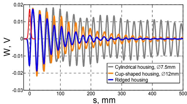
Figure 5: Longitudinal long range wakepotential.
