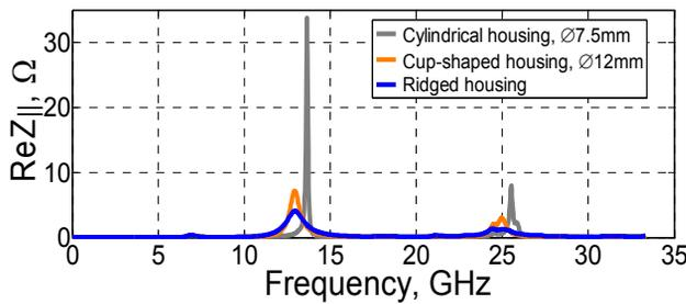
Figure 4: Real part of the longitudinal impedance.
