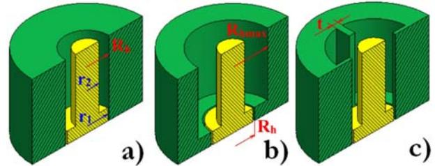
Figure 3: Housing modification for the BPM Button.
