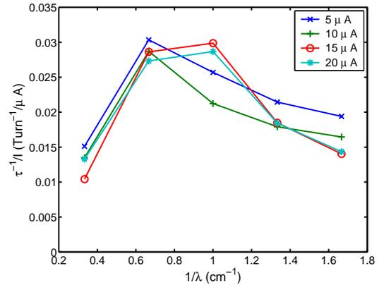
Figure 2: Amplitude growth rate for harmonics with the wavelength  $\lambda=0.6, 0.75, 1, 1.5,$  and  $3$  cm normalized to the peak beam current. The normalized growth rate shown for four different peak intensities:  $5, 10, 15$  and  $20 \mu\text{A}$ .
