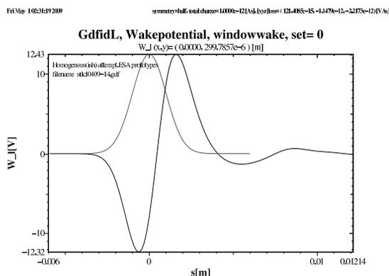
Figure 4: Longitudinal wakefields excited by a bunch of 1 mm in a complete collimator with closed jaws.
