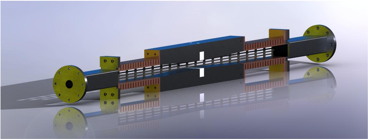
Figure 1: Impression of baseline full collimator structure with jaws open.
