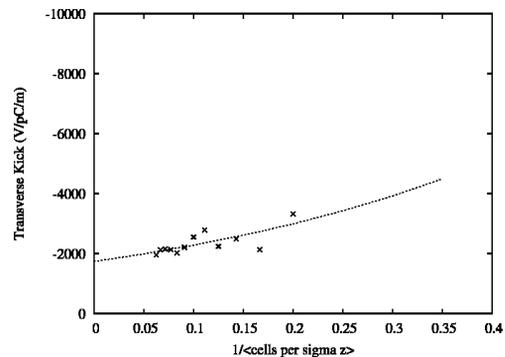
Figure 3: Convergence study for T480 collimator ‘6’, with 0.166 mrad taper angle, 1 mm bunch and small offset from the axis relative to the jaw size.
