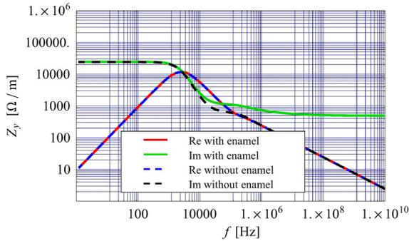
Figure 1: Calculation of the transverse impedance of a 0.5 mm thick dielectric layer ( $\epsilon_r = 5$ ) inside a 2 mm thick stainless steel pipe with 50 mm radius and 1 m length. For this rotationally symmetric structure the Burov-Lebedev formula was used [5].
