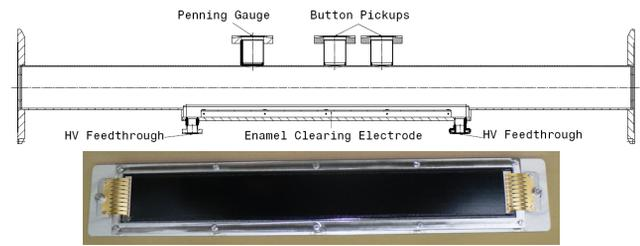
Figure 2: PS electron cloud experiment installed in SS84 comprising the enamel clearing electrode, a shielded Penning gauge and two shielded button-type pickups.
