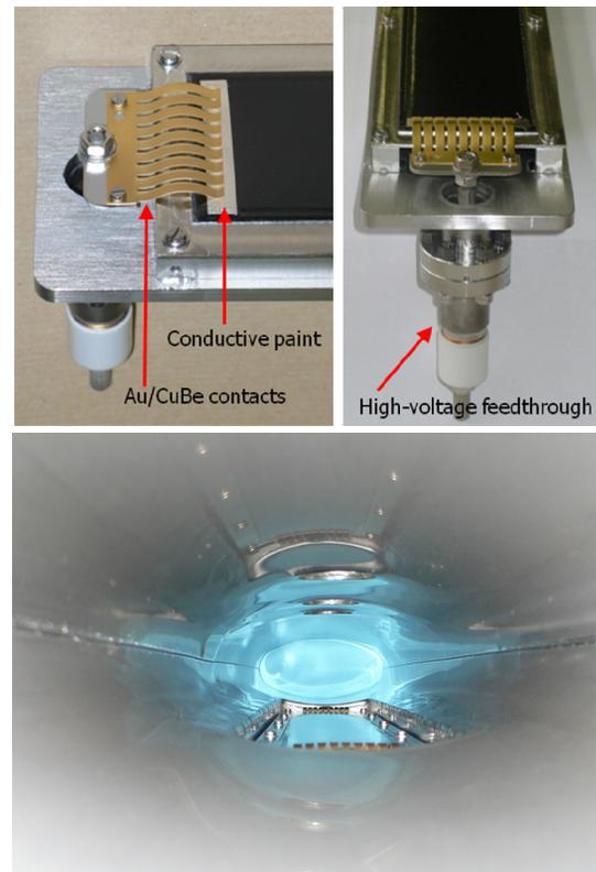
Figure 3: Enamel clearing electrode with high-voltage Au/CuBe contact fingers (top), downstream view into SS84 vacuum chamber showing the stripline electrode inside an antechamber (bottom).
