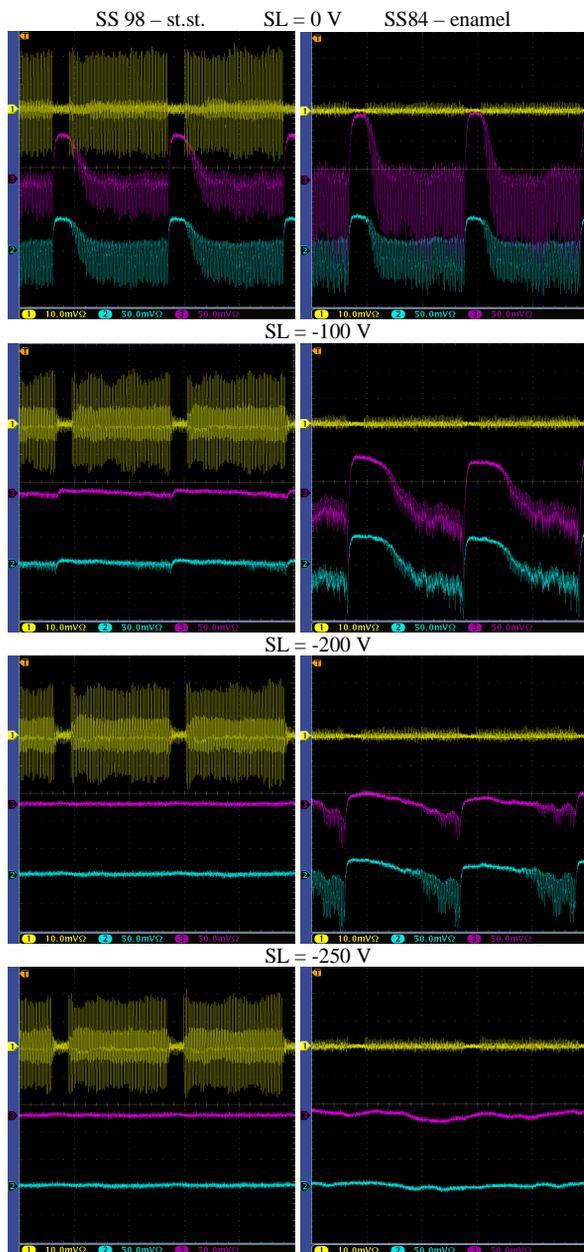
Figure 4: Measured electron cloud signals of the stripline electrodes (yellow) and the button pickups (magenta, cyan) during passage of the nominal LHC beam in SS98 (left column: stainless steel clearing electrode) and SS84 (right column: enamel clearing electrode) as a function of negative clearing voltages varied between 0 and -250 V.
