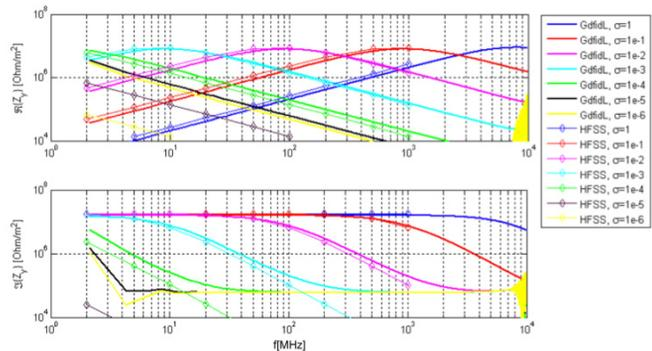
Figure 4: Comparison between GdFidL and HFSS [7] in the case of a round beam pipe with a radius of 2 mm, a length of 1 m, a thickness of 1 cm (with perfect conductor outside), for several values of conductivity: Real (upper) and imaginary (lower) part of the transverse impedance.
