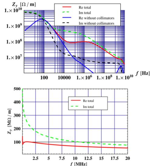
Figure 1: Vertical impedance at top energy after the squeeze (upper). Zoom between 8 kHz (1<sup>st</sup> unstable betatron line in the LHC) and 20 MHz (frequency limit of the transverse feedback).
