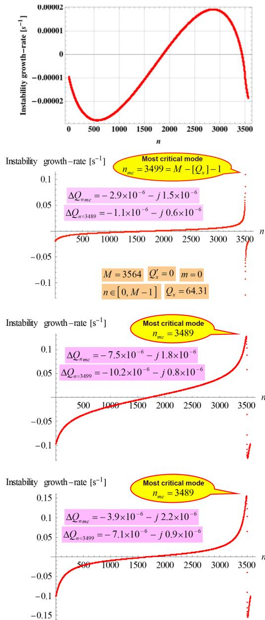
Figure 5: Instability growth-rate vs. the transverse coupled-bunch mode number  $n$  for the case of a round beam pipe with a radius of 2 mm and a length of 1 m: ceramic with a real dielectric constant of 5 and a resistivity of  $1 \Omega m$  (a), copper (b), graphite (c) and copper coated (with  $5 \mu m$ ) graphite (d). In all cases the thickness is 2.5 cm with vacuum outside.
