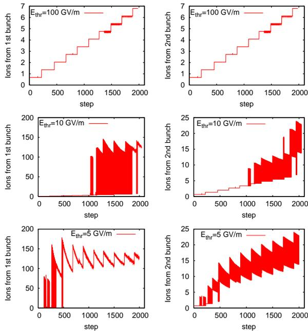
Figure 1: Ionization rates for first (left column) and second bunch (right column) with the threshold electric field for field ionization set to 100 (top row), 10 (middle row) and 5 GV/m (bottom row).
