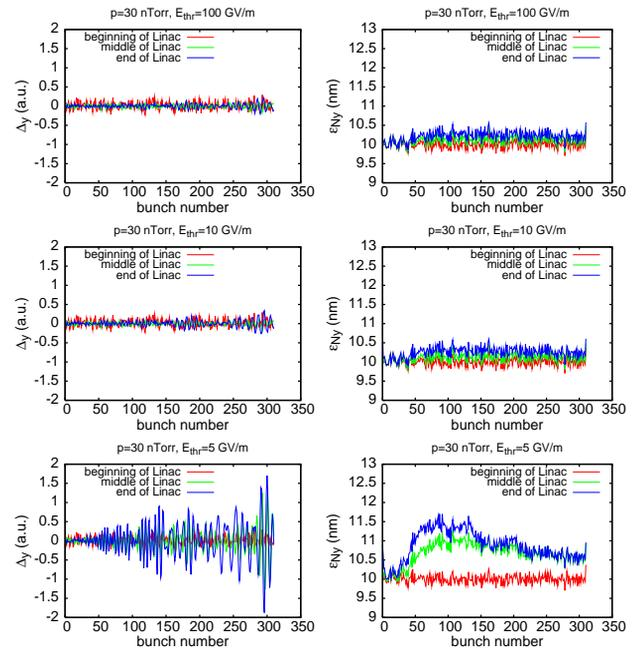
Figure 2: Bunch-by-bunch centroid vertical position (left column) and emittance (right column) at three different points along the linac (as labeled) with the threshold electric field for field ionization set to 100 (top row), 10 (middle row) and 5 GV/m (bottom row).
