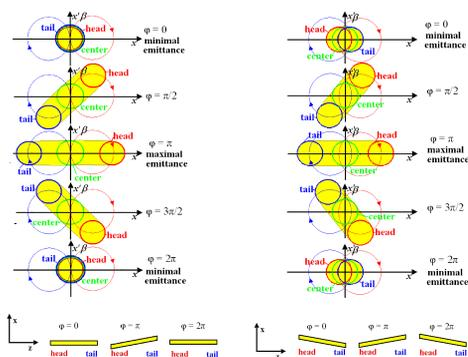
Figure 2: Phase diagrams for different betatron phases for particle belonging to different transverse bunch cross sections: head (red), center (green), and tail (blue). The emittance of the entire bunch is shown in yellow. Left and right hand sides show the cases without- and with- acceleration.
