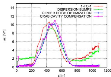
Figure 3: Emittance growth along the two-stage bunch compressor after the three correction schemes proposed.
