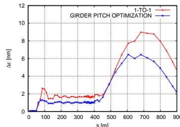
Figure 4: Emittance growth along the single-stage bunch compressor.
