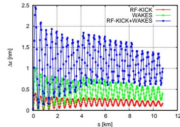
Figure 1: Emittance growth along the ILC main linac under the effects of RF and wakefield kicks induced by the couplers.
