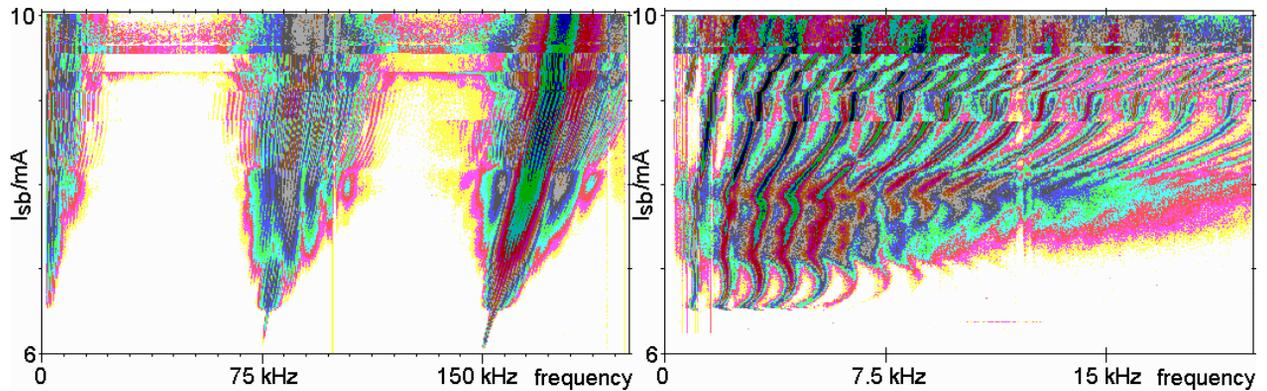
Figure 2: Spectral waterfall displays of the time dependent CSR-signals as a function of the single bunch current. The storage ring was operated with 4 sc IDs. The first time dependent signal shows up at 6.1 mA with a frequency ten and twenty times larger than the synchrotron frequency,  $F_{syn}=7.5$  kHz. The low frequency spectral content up to 20 kHz is shown on the right.
