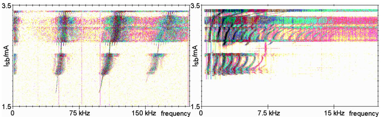
Figure 3: Waterfall displays like in Fig. 2, without the superconducting insertion devices. At 1.8 mA the first spectral lines appear at 44 kHz and 48 kHz. As in the previous figure the synchrotron frequency is 7.5 kHz. In both cases the low frequency signals ("bursts") have a higher threshold.
