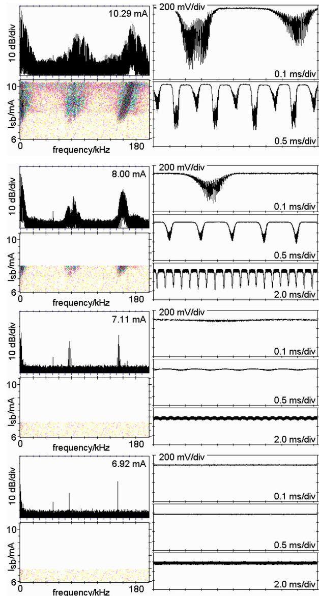
Figure 1: Time dependent CSR-signals for different single bunch currents (right) and the offline Fourier analysed spectra and the related spectral waterfall displays (left). Between 6.92 mA and 6.59 mA spectral lines are visible at multiples of 76 kHz. Below 6.59 mA only the noise related line at 52 kHz survives.
