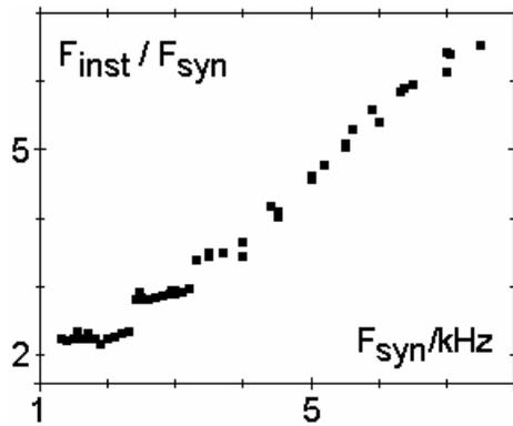
Figure 4: Normalized fundamental frequency of the first time dependent CSR-signal,  $F_{inst}/F_{syn}$ , as a function of bunch length (synchrotron frequency,  $F_{syn}$ ). This shows that well defined azimuthal modes are initially unstable. Measurements were taken without the sc IDs and the rms bunch length is  $\sim 13$  ps with  $F_{syn}=7.5$  kHz.
