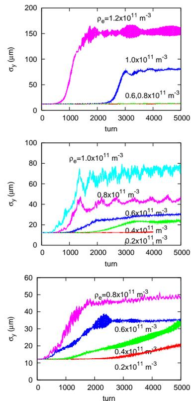
Figure 1: Growth of the vertical beam size caused by the electron cloud induced fast head-tail instability. Top is for  $\eta = 0$  m, centre is for  $\eta = 1$  m, and bottom is for  $\varepsilon_x = 0$ ,  $\eta = 1$  m.
