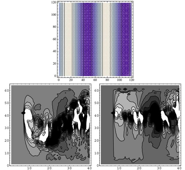
Figure 2: Wake field in  $x - z$  plane. Hor. and Vert. axes are  $z$  and  $x$ , respectively. The ontour displays  $F_y$ . (top) ordinary wake, (bottom left) drift space, (bottom right) in bending magnet.
