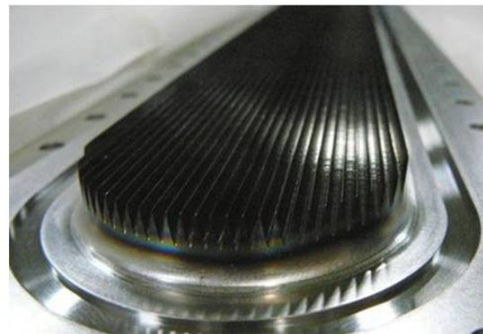
Figure 4: Triangular groove structure with TiN coating.
