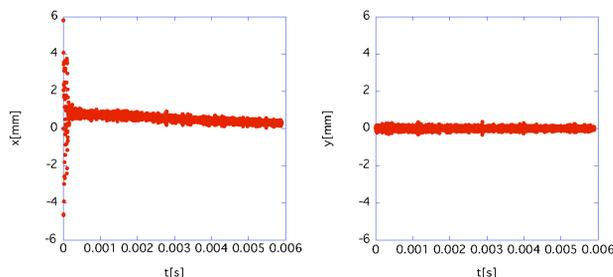
Figure 6: Simulation results at 300 kW beam operation with the space-charge effects. The left and the right figures show the horizontal and the vertical beam positions, respectively.
