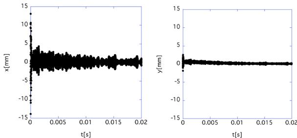
Figure 3: Transverse instability due to the kicker magnets without the space-charge effects at 300 kW operation in the RCS. The left and the right figures show the horizontal and the vertical beam positions, respectively. The chromaticity is corrected to zero in the entire energy.
