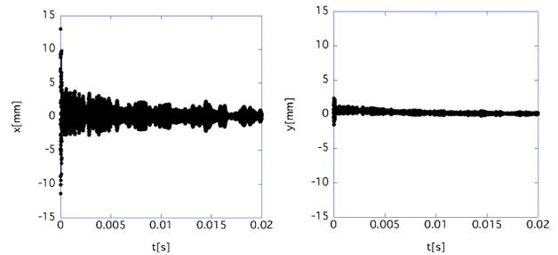
Figure 5: Transverse instability due to the kicker magnets without space-charge effects at 300 kW operation in the RCS. The left and the right figures show the horizontal and the vertical beam positions, respectively. The chromaticity is corrected to zero only at the injection energy.
