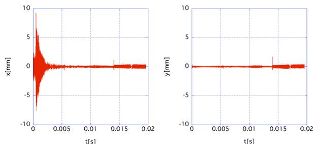
Figure 8: The measurement results for 300 kW beam operation. The left and the right figures show the horizontal and the vertical beam positions, respectively.
