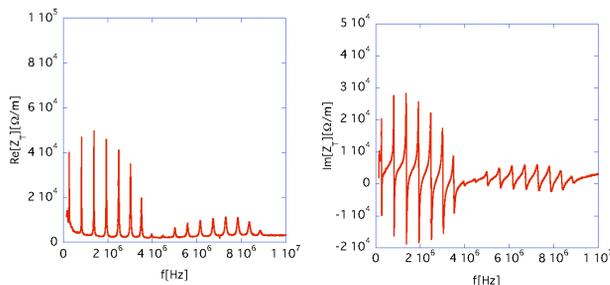
Figure 1: The measurement results of a kicker impedance of the RCS. The left and the right figures show the real and the imaginary parts, respectively. The total number of the kicker magnets  $n_k$  is eight in the RCS.
