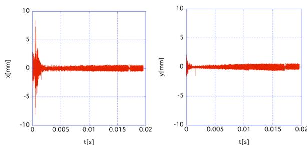
Figure 7: The measurement results for 100 kW beam operation. The left and the right figures show the horizontal and the vertical beam positions, respectively
