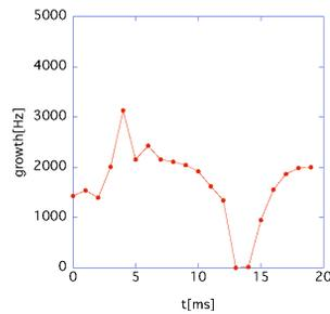
Figure 2: Horizontal instability due to the kicker magnets at 0.6 MW beam operation in the RCS. The chromaticity is corrected to zero in the entire energy. The growth rate will be halved at 300 kW beam operation.
