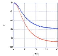
Figure 4: The behavior of chromaticity along time axis. The red and the blue lines show the horizontal and the vertical chromaticity, respectively.
