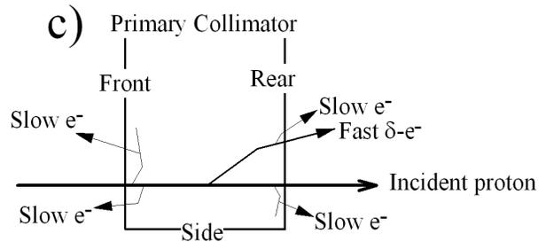
Figure 2: Patterns as ways to hit the primary collimator with an incident proton.
