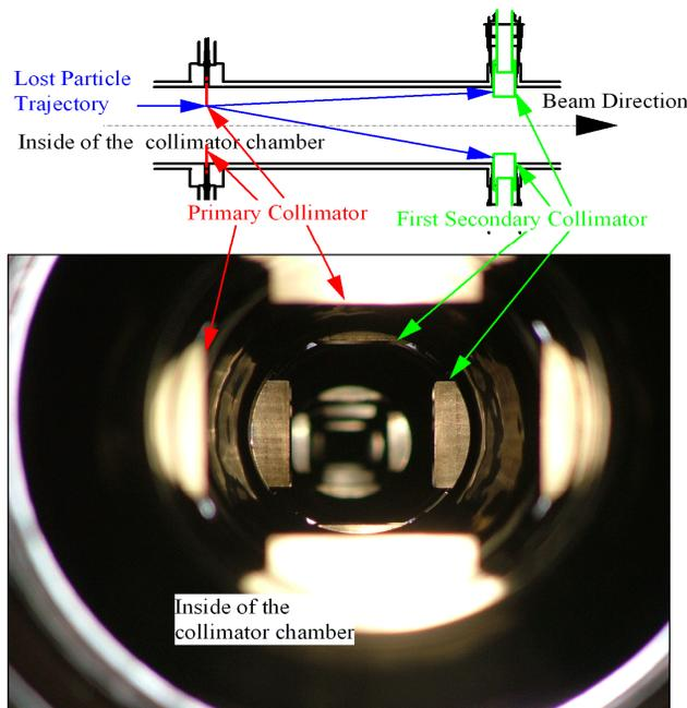
Figure 4: Inside of the collimator chamber.
