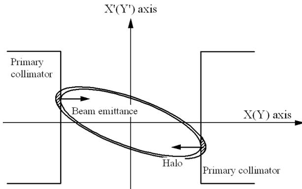
Figure 3: The angle of the lost (halo) particle.
