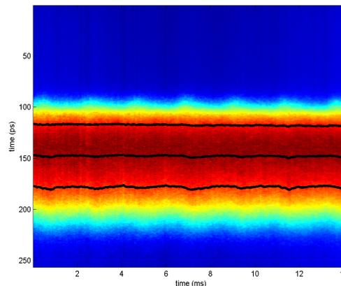
Figure 4: Streak camera image of single bunch longitudinal current distribution in correspondence of THz bursting.
