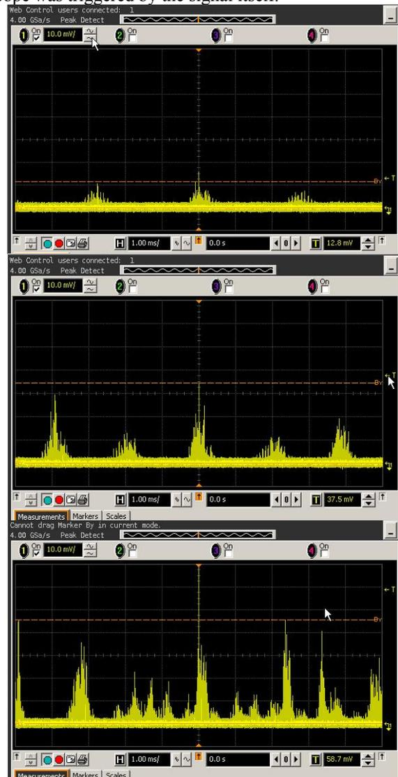
Fig. 3: Oscilloscope traces of the signal from the Schottky Diode showing the onset of the THz bursts at 1.9 mA (top), at 3 mA (middle) and a chaotic series of bursts at 5.2 mA (bottom).
