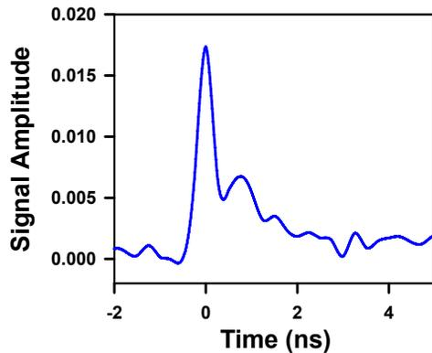
Figure 2: Typical signal from DXP-12 for the THz emission generated by a single bunch in the diamond storage ring. The signal amplitude is in Volts.
