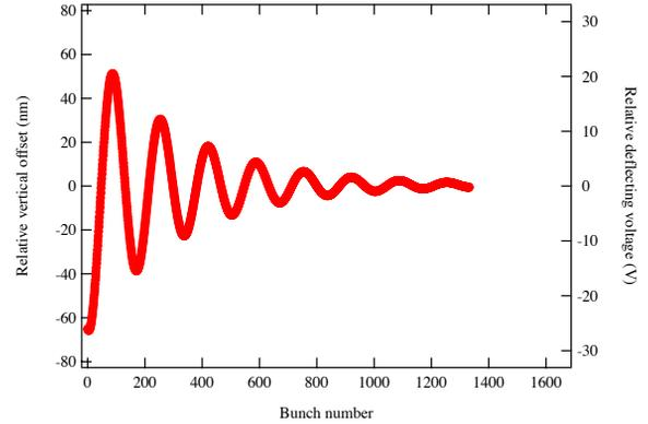
Figure 1: Calculation of the relative transverse voltage and offset along the bunch train for the parameters shown in Table 1. The dipole mode is tuned to the one revolution frequency away from the second harmonic of the RF frequency. The value of  $R/Q=1$  Ohm.
