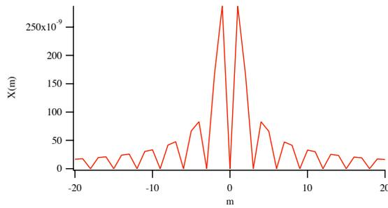
Figure 2: Shows the size variation of the transverse transient as a function of the deflecting cavity tuning,  $m$ . Here  $m$  is assumed to be an integer and the quality factor of the cavity,  $Q$ , is assumed to be very large. Notice that the largest peak occurs at  $m = 1$ .
