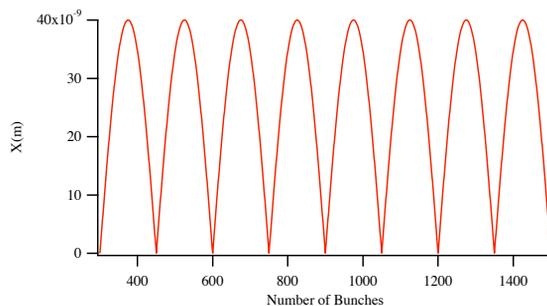
Figure 3: This shows the size of the transverse transient as a function of the number of bunches in the bunch train.
