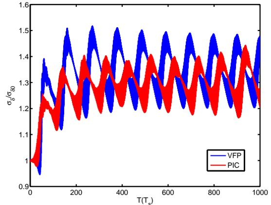
Figure 1: A comparison between VFP and PIC codes using the impedance of the SLC damping ring [4]. The number of macro particles is chosen to be the same as the number of grid points in the VFP solver.
