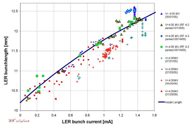
Figure 2: LER bunch length as a function of a bunch current measured in multi-bunch regime at different RF station combination and simulated (solid line).
