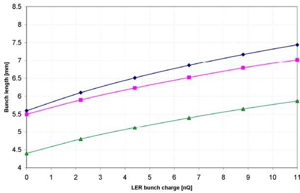
Figure 5: Bunch lengthening as a function of a bunch charge in Super-B for LER at different RF: green line for 12 MV, pink line for 8 MV and blue line for 6 MV.
