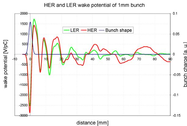
Figure 4: HER (red) and LER (green) wake potentials of a 1 mm bunch, which were used as quasi-Green's functions to calculate the bunch lengthening.
