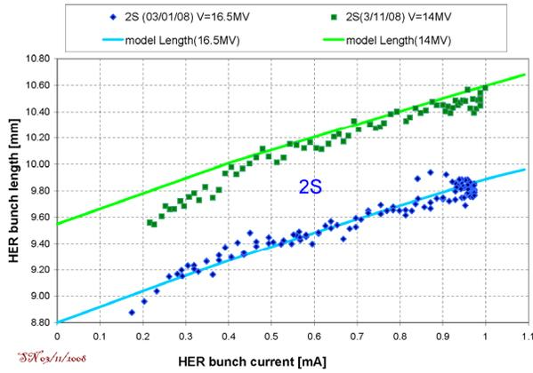
Figure 3: Measured and simulated (solid lines) HER bunch length as a function of a bunch current at the 2S for two different RF voltages: 16.5 MV (blue diamond) and 14 MV (green squares). Measurements were done in multi-bunch regime.
