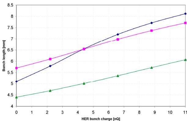
Figure 6: Bunch lengthening as a function of a bunch charge in Super-B for HER at different RF: green line for 20 MV, pink line for 12 MV and blue line for 8 MV.
