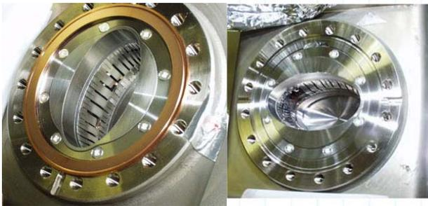
Figure 4: Discharges in shielding fingers of vacuum valves.
