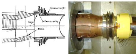
Figure 1: Vertex bellows in interaction region.
