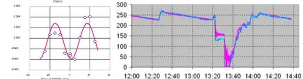
Figure 2: Left plot: Modulation of heating by changing the phase of the electron beam. The curve corresponds to 5.4 GHz. Right plot: History correlation of the amplitude of the 5.59 GHz mode (blue line) and heating power, calculated from the bellows temperature.
