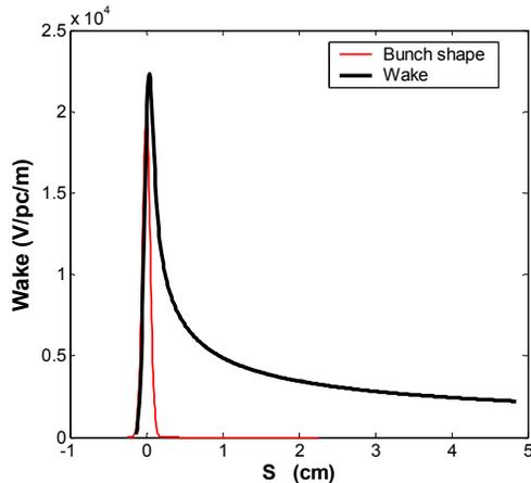
Figure 1: Transverse Wake convoluted with 0.5mm Gaussian bunch.
