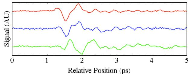
Figure 4: measured signal after the initial pulse (red) is propagated through 2.5 cm (blue) and 10 cm (green) 5 mm diameter copper waveguide.
