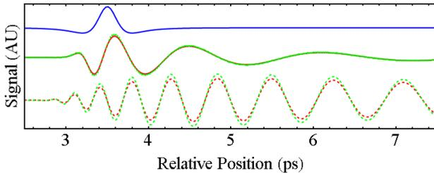
Figure 2: Propagation of a pulse (blue) through 50 cm of 5 mm (middle) and 2 mm (bottom) diameter waveguide with (red) and without (green) attenuation.
