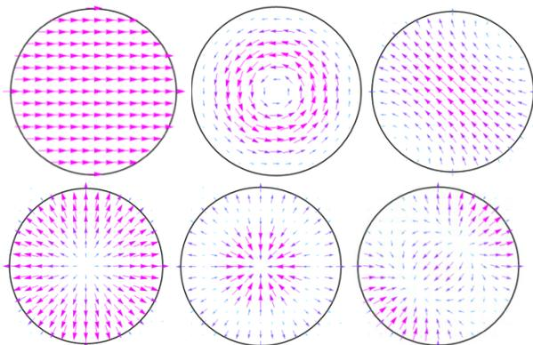
Figure 5: Electric field patterns for the incoming laser pulse, TE01, TE11, TM01, TM02 and TM11 modes.
