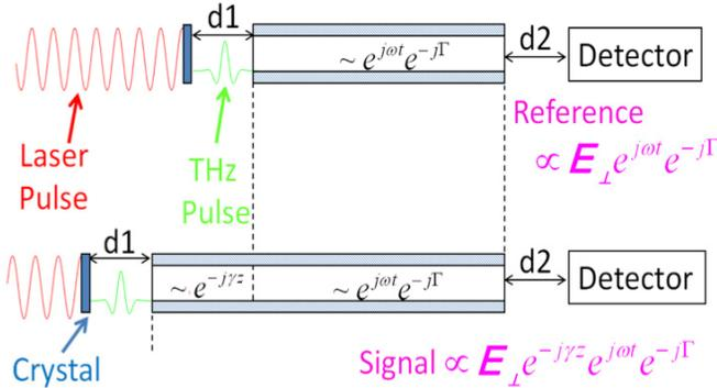
Figure 1: Scaling of propagation factors as the waveguide length is increased.
