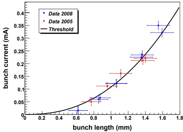
Figure 5: The observed bursting stable threshold as function of bunch current and bunch length. The black curve shows the fit to the microbunching theory.
