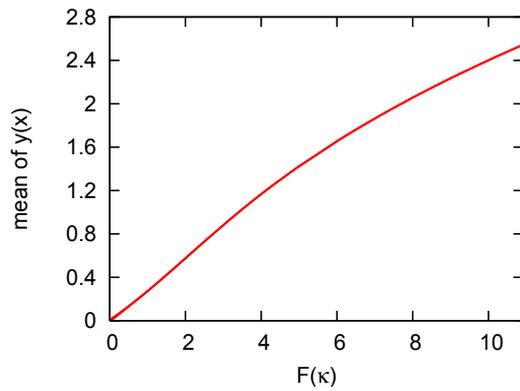
Figure 2: The dependence of the mean of the electron distributions versus  $F(\kappa)$ . For a constant bunch length,  $F(\kappa)$  is proportional to the bunch current.
