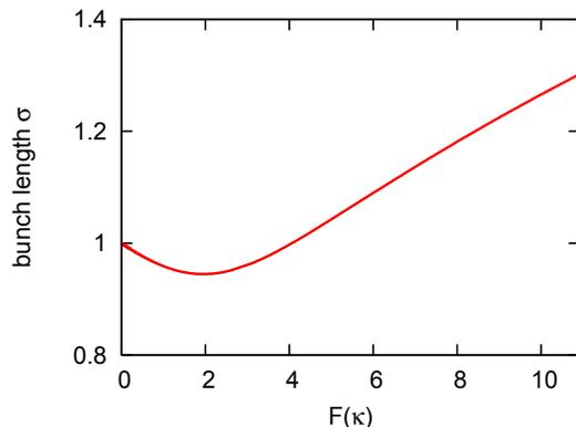
Figure 3: The bunch length  $\sigma$  versus  $F(\kappa)$ . The bunch shortens till a minimum at  $F(\kappa) = 1.94$  and increases again.
