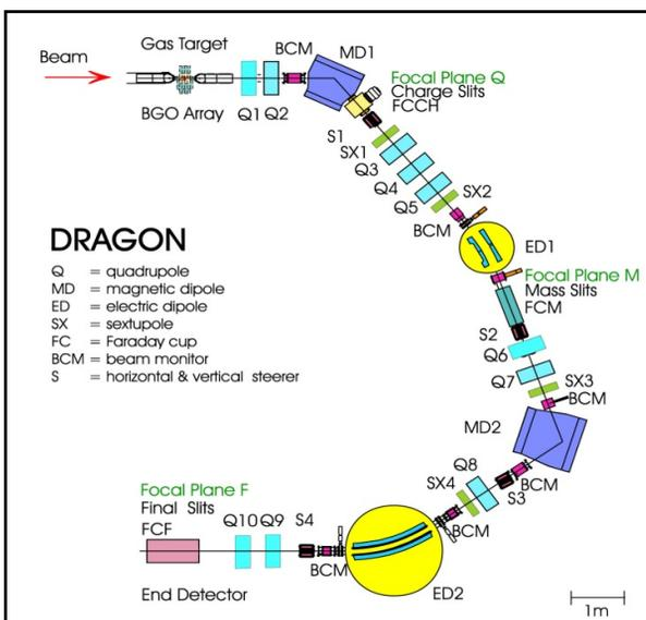
Figure 6: The DRAGON spectrometer. This is designed to study low energy charge particle capture reactions at energies relevant to astrophysical situations. The spectrometer detects the rare capture events and strongly suppresses the intense radiation background effects from the incident RIB.
