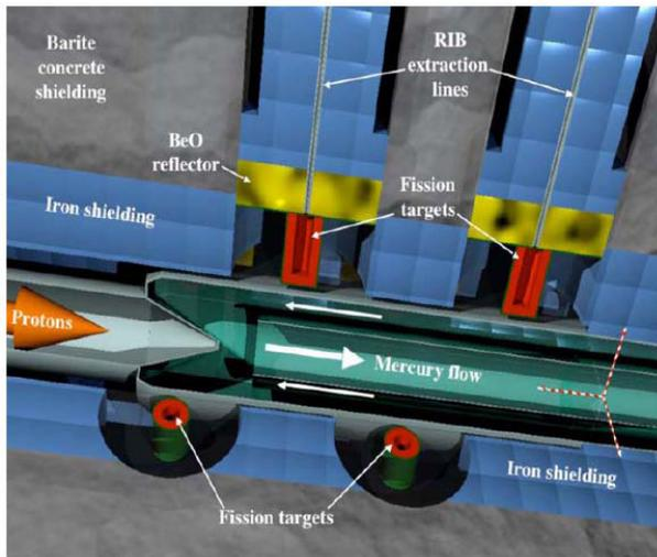
Figure 5: The EURISOL 4MW target
