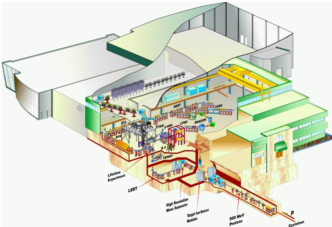
Figure 3: The RIB facility at TRIUMF uses the 500 MeV cyclotron 100  $\mu$ A proton beam to irradiate ISOL targets.
