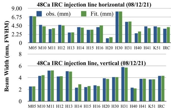
Figure 5: Result of least square fitting of beam widths on IRC injection line. A 345-MeV/nucleon  $^{48}\text{Ca}$  beam was analyzed.
