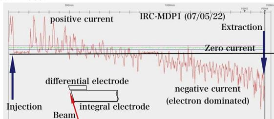
Figure 3: Effect of secondary electrons observed with IRC-MDP1.
