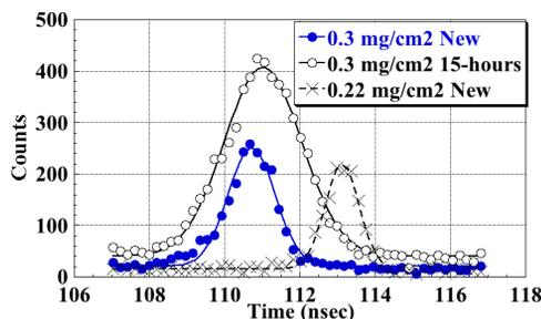
Figure 2: Longitudinal beam width measured by plastic scintillators.
