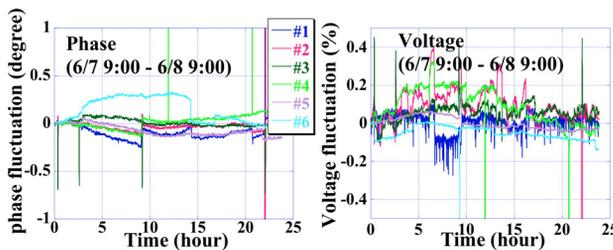
Figure 4: Results of RILAC Stability Test
