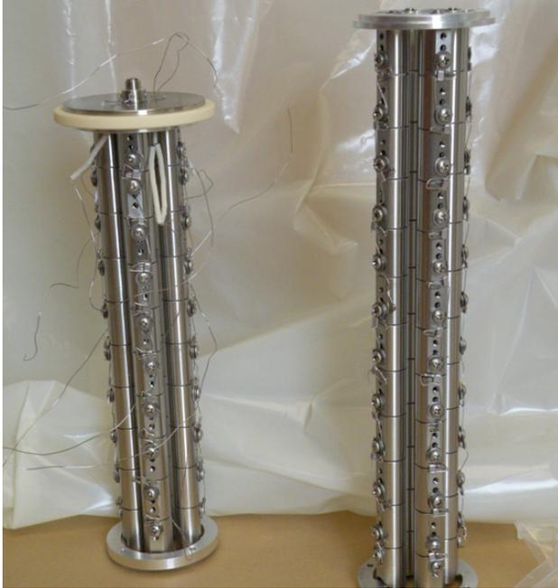
Figure 5: Two stage RFQ cooler for maintaining small beam size as helium gas in pumped away in three differential pumping stages. MicroRFQ seen on top flange of left assembly maintains focusing forces through the differential pumping isolator. Left RFQ is 30 cm long for scale.
