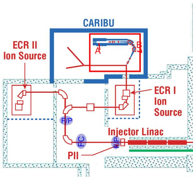
Figure 2: CARIBU floor plan showing the major elements. The  $^{252}\text{Cf}$  source is located at position 'A'. The high resolution isobar separator is mounted on the CARIBU platform at position 'B'. "F/P" refers to weak beam diagnostics with profile and ion counting ability, whereas "FC" refers to ion counting only.
