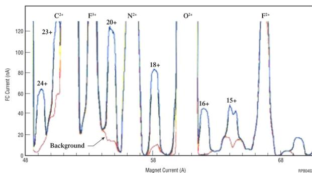
Figure 7: Charge state distribution for  $^{133}\text{Cs}^{1+}$  beam injected into the ECR CB ion source. The red plot shows the background with no 1+ beam going into source.
