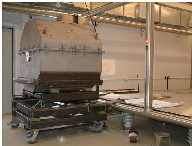
Figure 8: CARIBU shield cask shown in position to be rolled onto the CARIBU HV platform.
