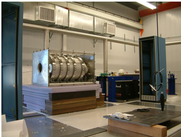
Figure 9. CARIBU High voltage platform assemble showing current status as of this conference.
