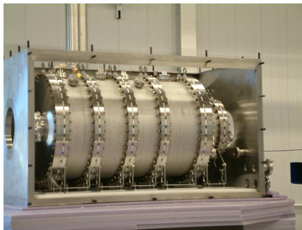
Figure 4: Assembled gas catcher mounted in isolation box. In operation both gas catcher and box are filled with one quarter to one half atmosphere helium. The enclosing rectangular box is 1.47 m long.
