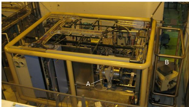
Figure 6: The ECR charge breeder ion source (A) mounted on its HV platform. The switching magnet directing stable beams for development and setup is seen on the right hiding the 1+ source (B).
