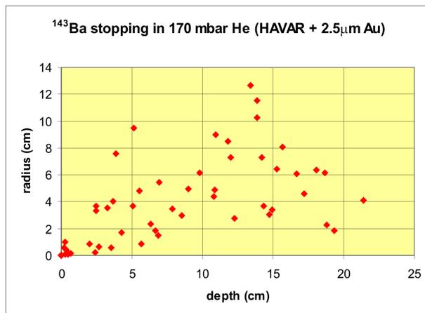
Figure 3: Ion stopping distances in 170 mbar helium gas after initial slowing in a gold degrader foil. Lifetime studies of various foils indicate that aluminum is a better degrader material and will be used instead of gold.
