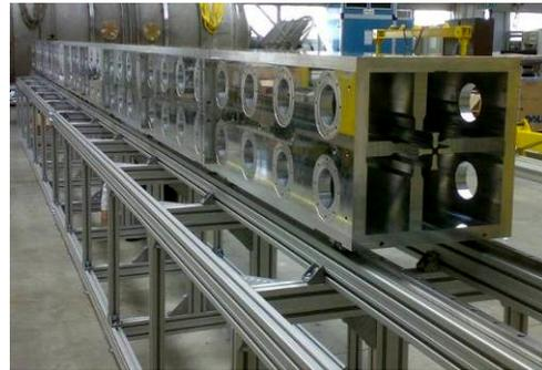
Figure 6: Full scale low power model of IFMIF RFQ.
